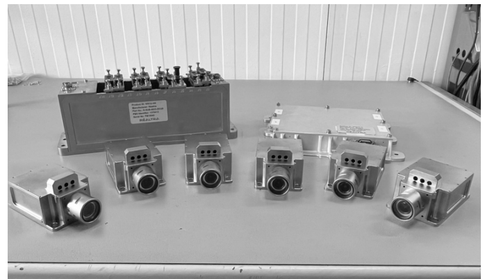
VIKI – Integrated Independent Video Kit for use on the Ariane 6 launch vehicle
